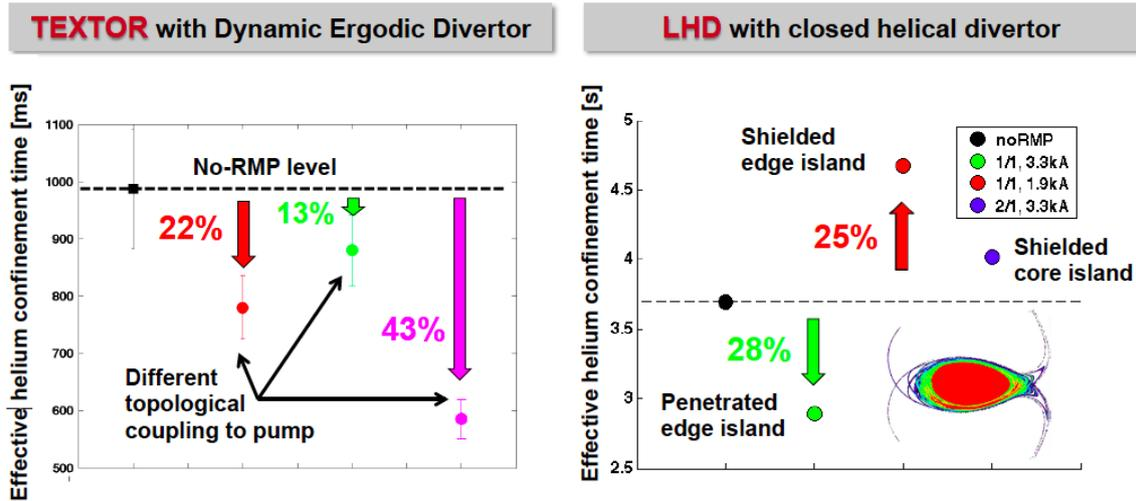
FIG. 2: Comparison of  $\tau_{p,He}^*$  at TEXTOR (left side) and LHD (right side). For TEXTOR three different orientations of the 3-D boundary with respect to the ALT-II limiter pump device is shown. For LHD, results for a penetrated edge island case (green) is compared to the noRMP situation in black and two RMP cases where island healing occurred.
