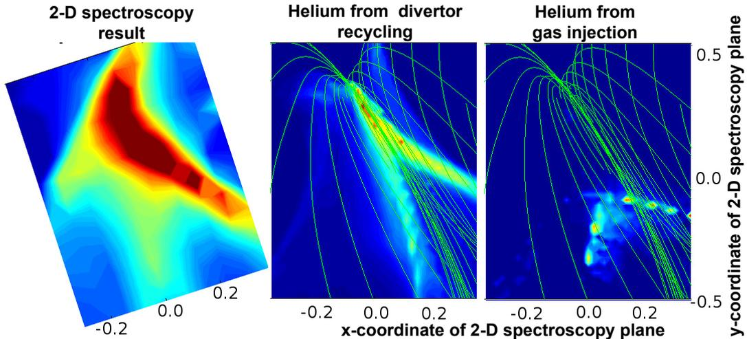
FIG. 4: 2-D images of the neutral helium emission at  $\lambda = 667.8\text{nm}$  from a new 2-D imaging spectroscopy (left side) and from synthetic modeling with EMC3-EIRENE[4]. Fueling from divertor recycling was compared to fueling solely from the gas injection.
