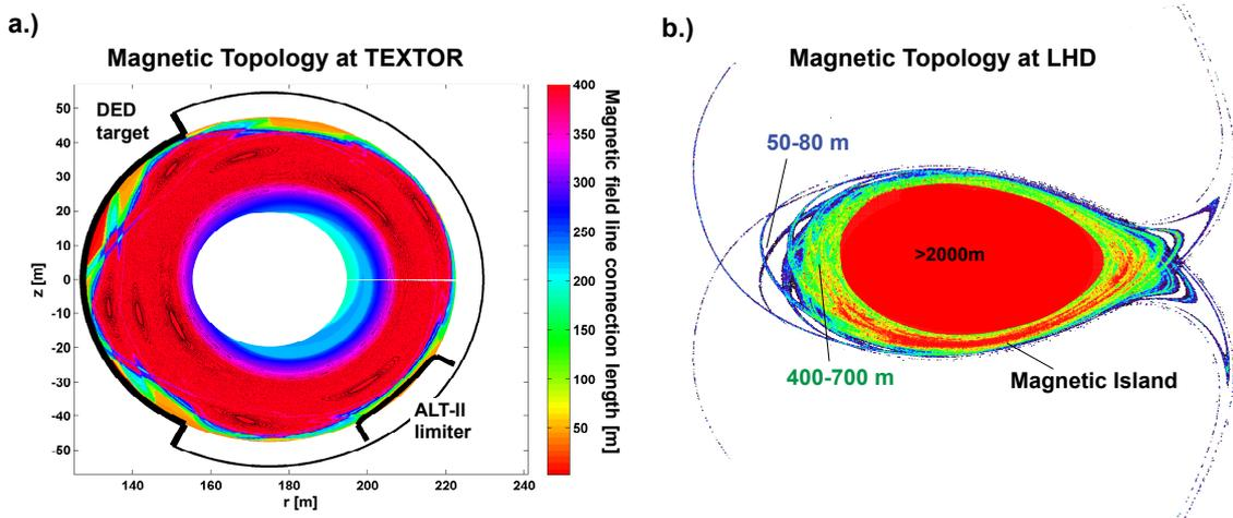
FIG. 1: Magnetic topologies addressed at TEXTOR-DED (figure a, left side) and LHD (figure b, right side) showing the magnetic wall to wall connection length  $L_c$ .
