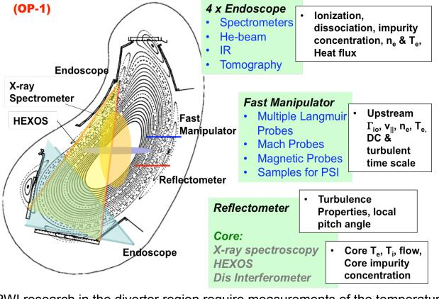
PWI research in the divertor region require measurements of the temperature in the plasma edge and of the concentration and distribution of different impurities, in combination with modelling of impurity transport.
