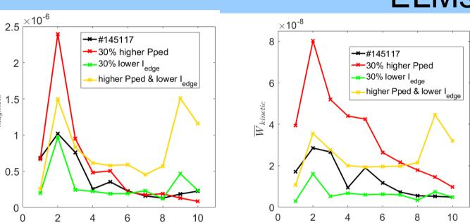
Sufficiently high edge current is essential for plasma to saturate to QHmode while high pressure pedestal is important for having ballooning mode
