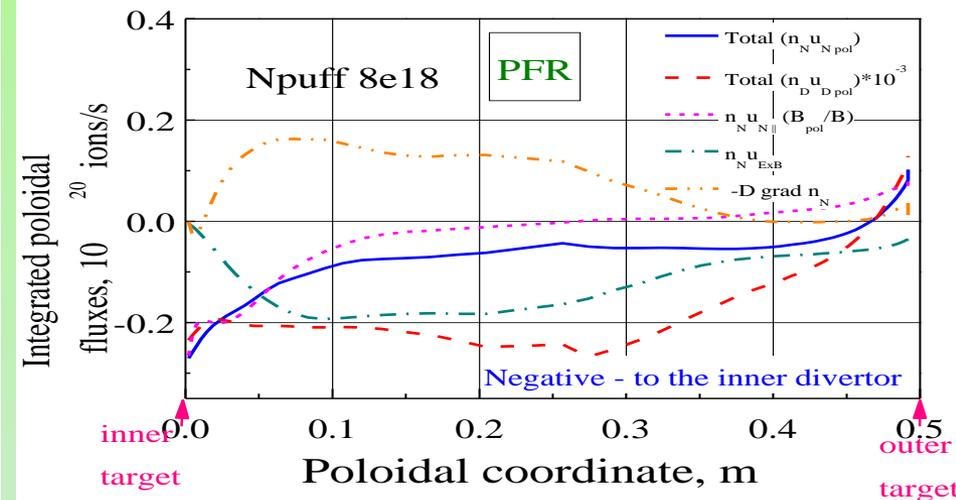
As a result, nitrogen retains at inner target and leaks at outer target
