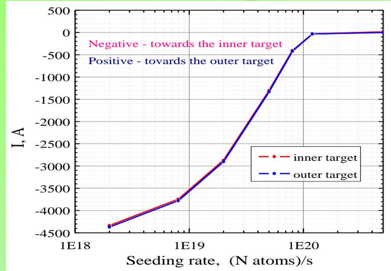
PS current dominates in the SOL and in PFR, however, directions are opposite, and SOL and PFR parts almost cancel each other. Sign of the net current is defined by thermoelectric current.
