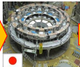
Lower EF Coils (100 tons)
