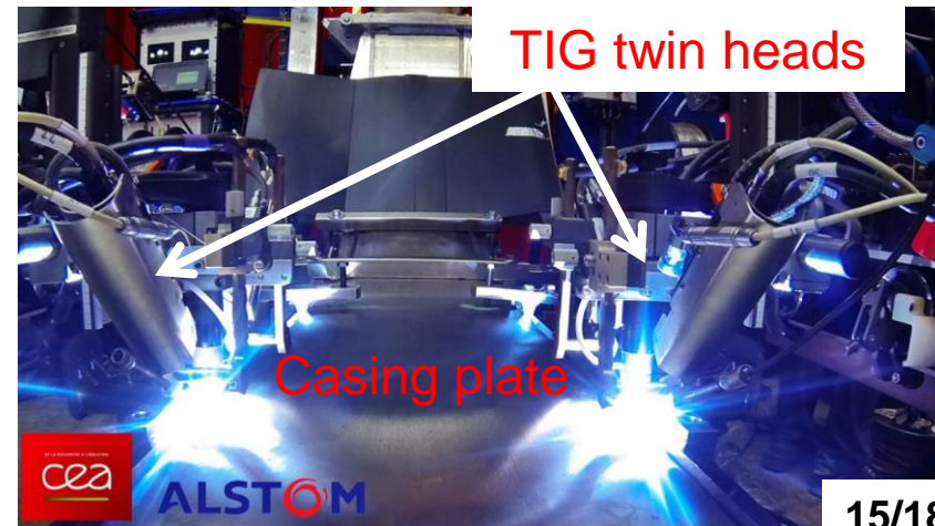
Longitudinal welding by TIG twin heads
