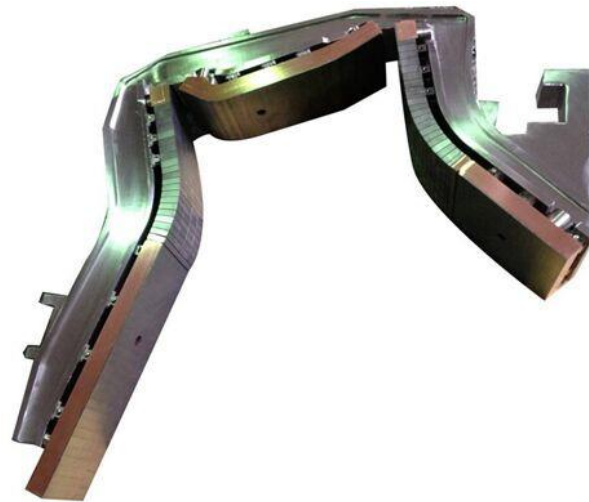
FIG. 3. Assembled set of PFC/CB, consisting of inner and outer targets and dome, with 9 monoblock plasma-facing units and 3 flat-type plates.
