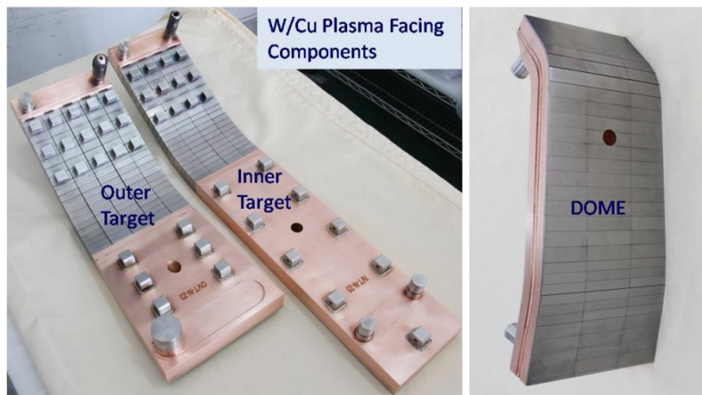
FIG. 4. W/Cu PFCs for EAST upper divertor.
