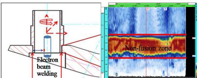
Improving NDT for welding seam of tube-plate joints inspection
