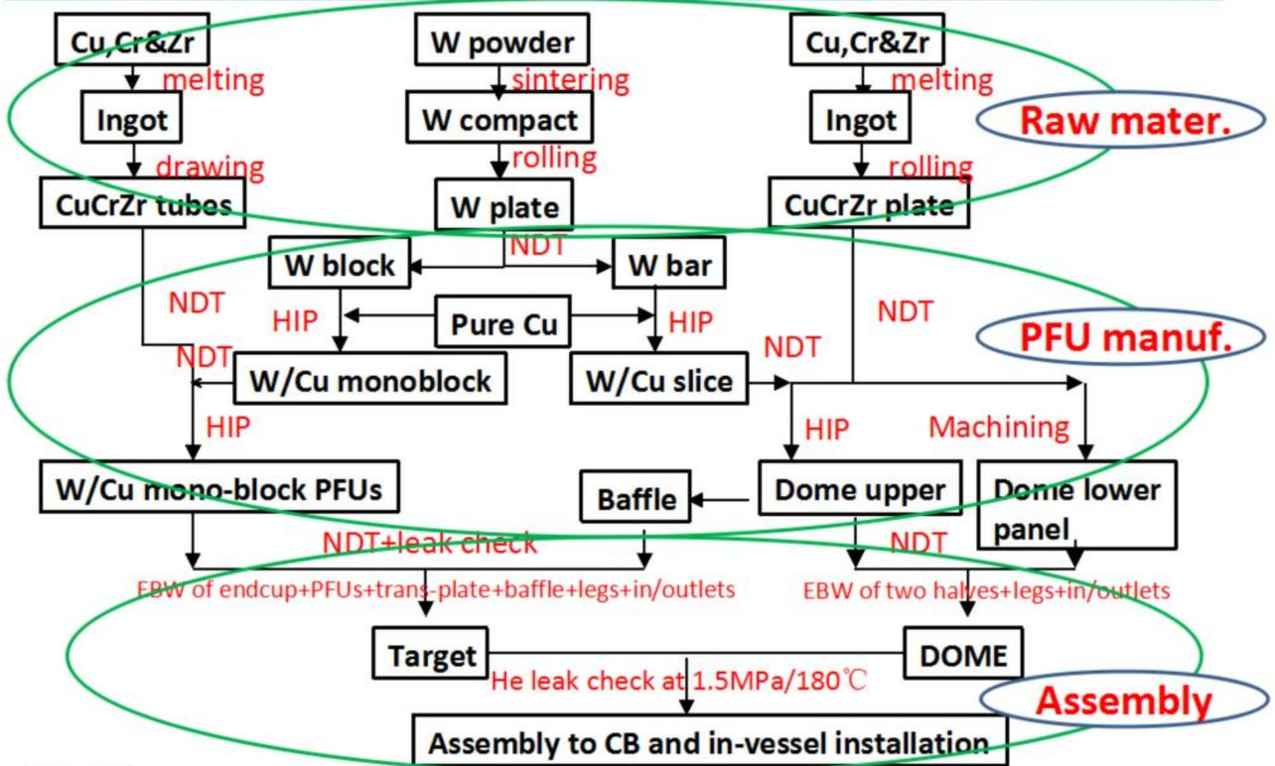
HIP technology is widely used in the bonding of W/Cu and Cu/CuCrZr.
