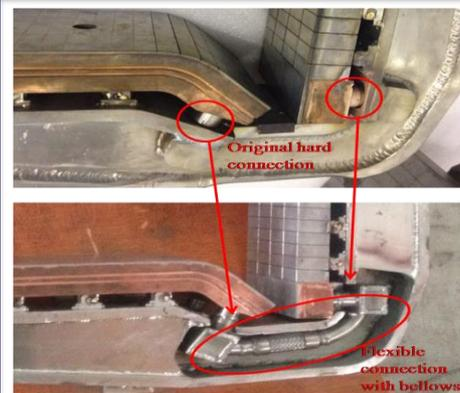
Optimizing cooling tube connection using bellows
