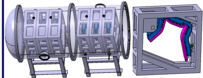
Performing baking and high pressure helium leak check on whole assembled div. modules
