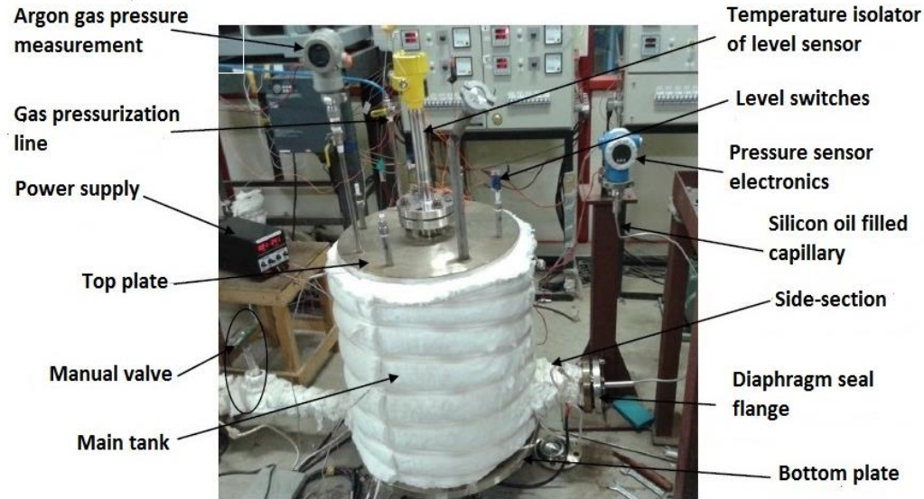
Level and pressure sensors installed on main tank
