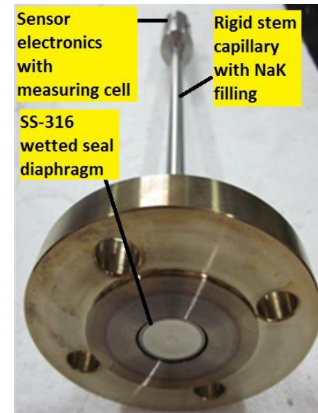
NaK filled capillary based customized pressure sensor
