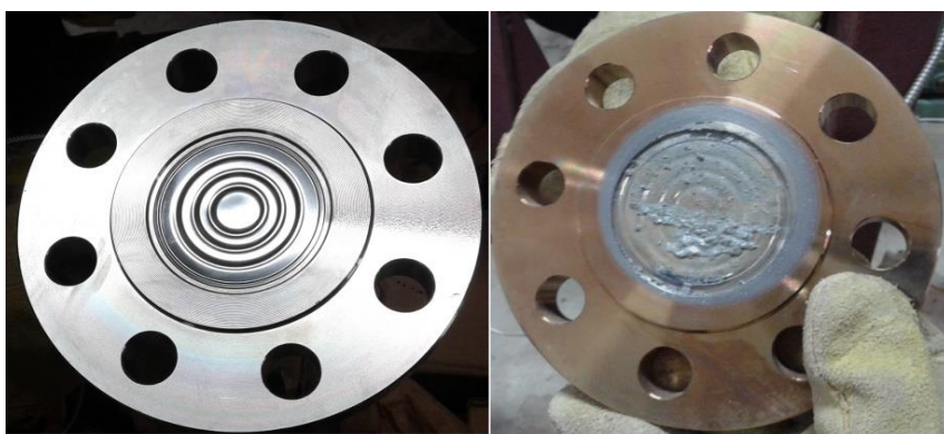
Condition of diaphragm seal after exposure to liquid lead
