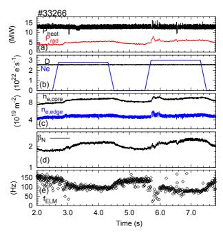
Figure 4: Time traces of (a) heating (black) and radiated (red) power, (b) fuelling waveforms for deuterium (black) and neon (×10, blue), (c) core (black) and edge (blue) line integrated densities, (d) normalised global beta and (e) ELM frequency for discharge #33266.
