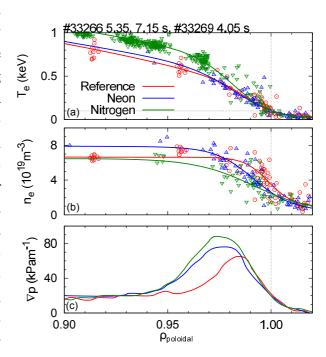
Figure 5: Profiles of (a) electron temperature (b) electron density and (c) the total pressure gradient for reference (red) neon seeded (blue) and nitrogen seeded (green) phases in two discharges (#33266, reference and neon and #33269, nitrogen).
