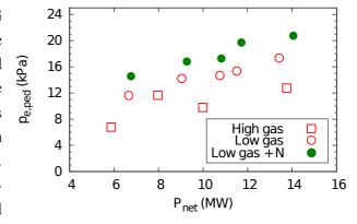
Figure 1: Pedestal top pressure as a function of applied heating power for high gas (red squares), low gas (red circles), and low gas with impurity seeding (filled blue circles).
