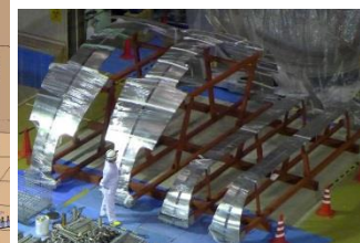
VV Thermal Shield (28 tons)
