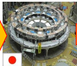
Lower EF Coils (100 tons)
