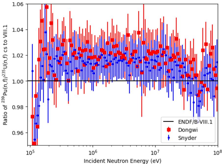
Background: Could be a thermal background that cannot be easily simulated (unknown how much water was in concrete). **Added 0.75% systematic unc.** which is a mid-sized estimate of the effect.
