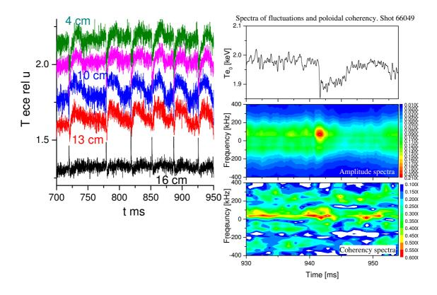
A sawteeth crash causes the rise of  $T_e$  and  $n_e$  outside inversion radius  $r_s$ . The reflectometer data shows enhanced level of the turbulence during 1-2 ms after the crash (at frequency 40-120 kHz) outside  $r_s$ .  $T_e$  and  $n_e$  decays fast.
