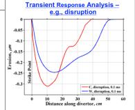
Divertor surface erosion profile after the impact of a disruption; W and C surfaces; ITER divertor. HEIGHTS code package analysis. Erosion due to vaporization is serious but not strongly material-dependent. The W-alternative materials will not have fundamentally different transient responses.
