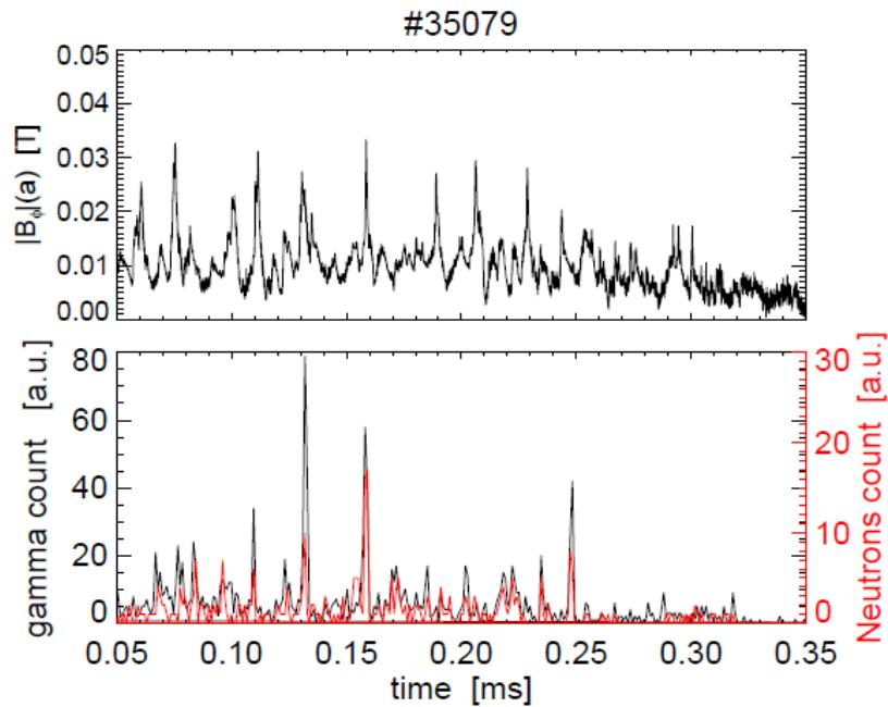
Bursty generation of DD fusion neutrons and  $\gamma$  rays
