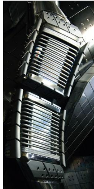
FAIT antenna (#4.5) Field-aligned, transforming \eta_{\text{heat}} \sim 80\% , S_{\text{excite}} \sim 0.12 \text{ m}^2
