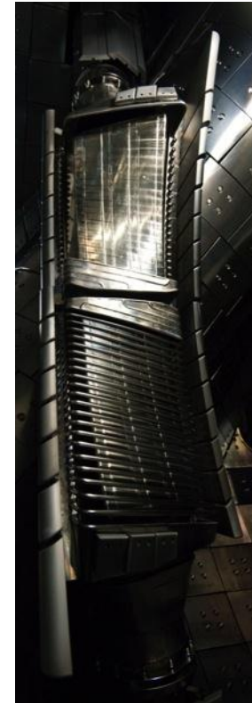
FAIT antenna (#4.5) Field-aligned, transforming \eta_{\text{heat}} \sim 80\% , S_{\text{excite}} \sim 0.12 \text{ m}^2
