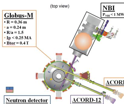
Main modeling techniques: NUBEAM, 3D fast ion tracking algorithm + Solution of Boltzmann kinetic equation + NPA LOS sim. Secondary techniques: EFIT, Double.
