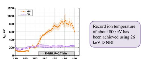
However, fast ion losses are much higher + additional channel of losses - sawtooth oscillations.
