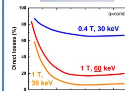
NUBEAM modeling simulations show that for 60 keV beam total losses won't exceed 50% and neutron rate will be increased more than two orders of magnitude ( $\approx 5 \cdot 10^{13}$  n/s).
