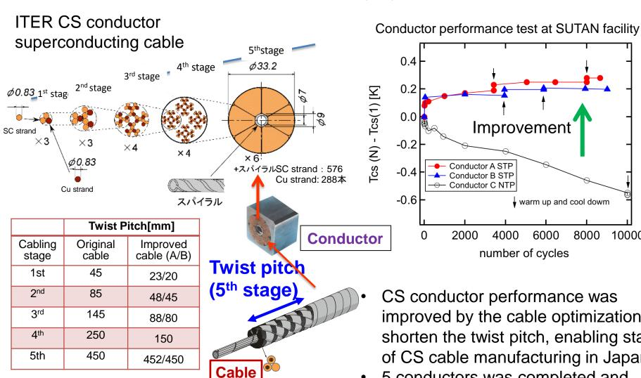
Twist pitch: the longitudinal length necessary for one twist
