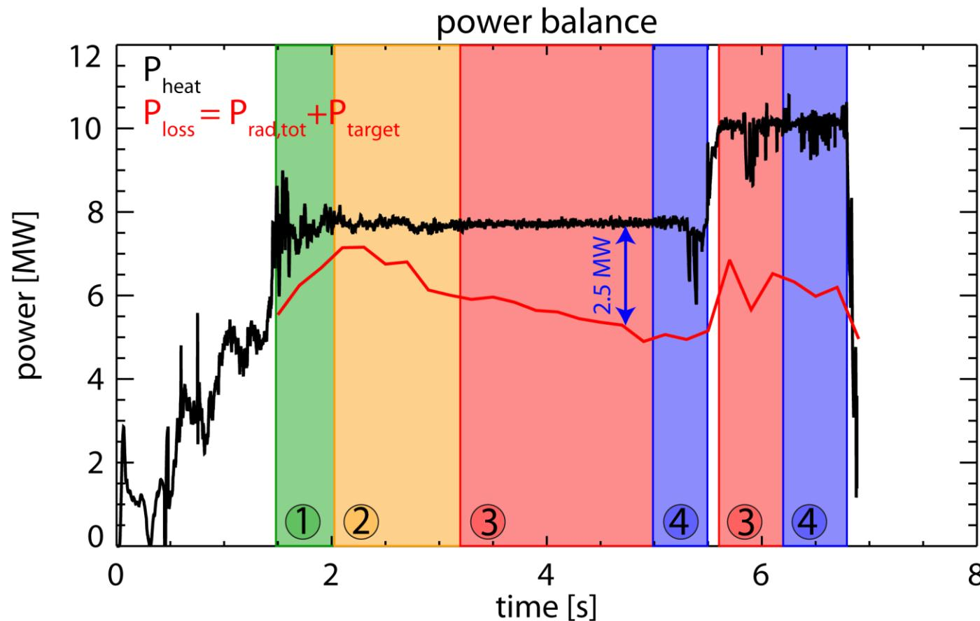
Stagnation of core density build-up due to fuelling limit (source shifts to SOL)
