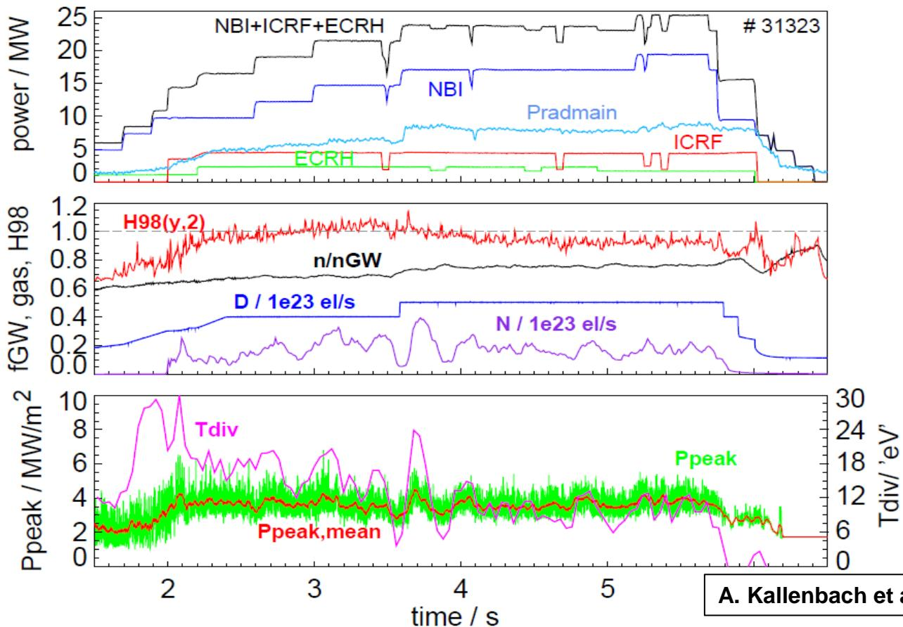
Feedback controlled N-seeding:  $q_{div} < 5 \text{ MW/m}^2$  at  $P_{heat} = 23 \text{ MW}$
