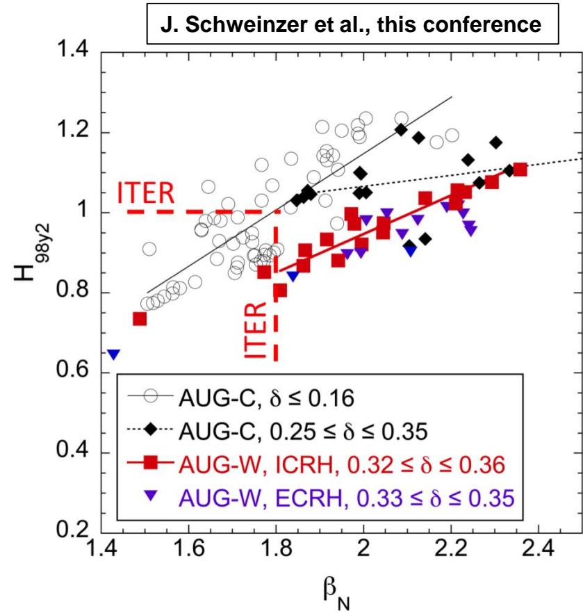
Due to changed operational window, target can only be met at higher  $\beta_N$
