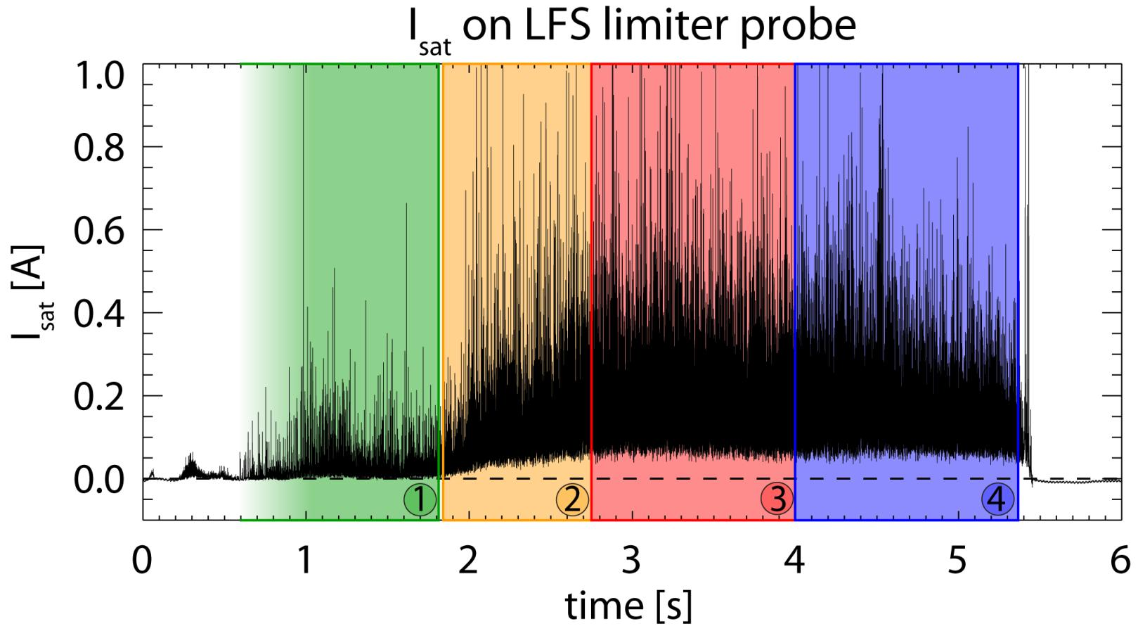
Stagnation of core density build-up due to fuelling limit (source shifts to SOL)
