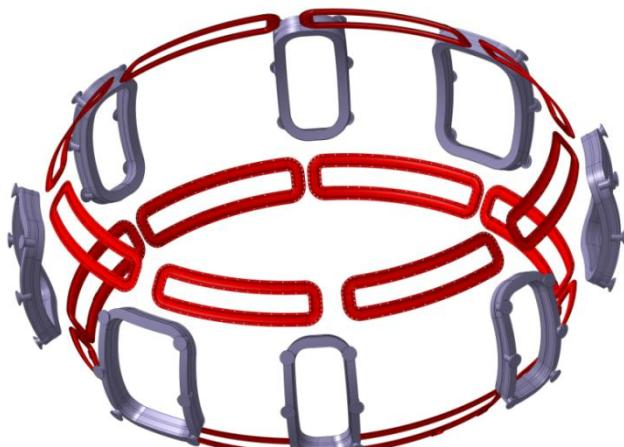
New: rotating fields up to 150 Hz, continuous poloidal phase scan at constant  $n$
