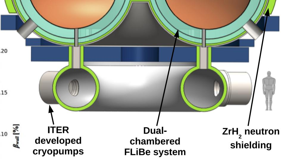
FliBe immersion blanket system allows for sufficient TBR of 1.125
