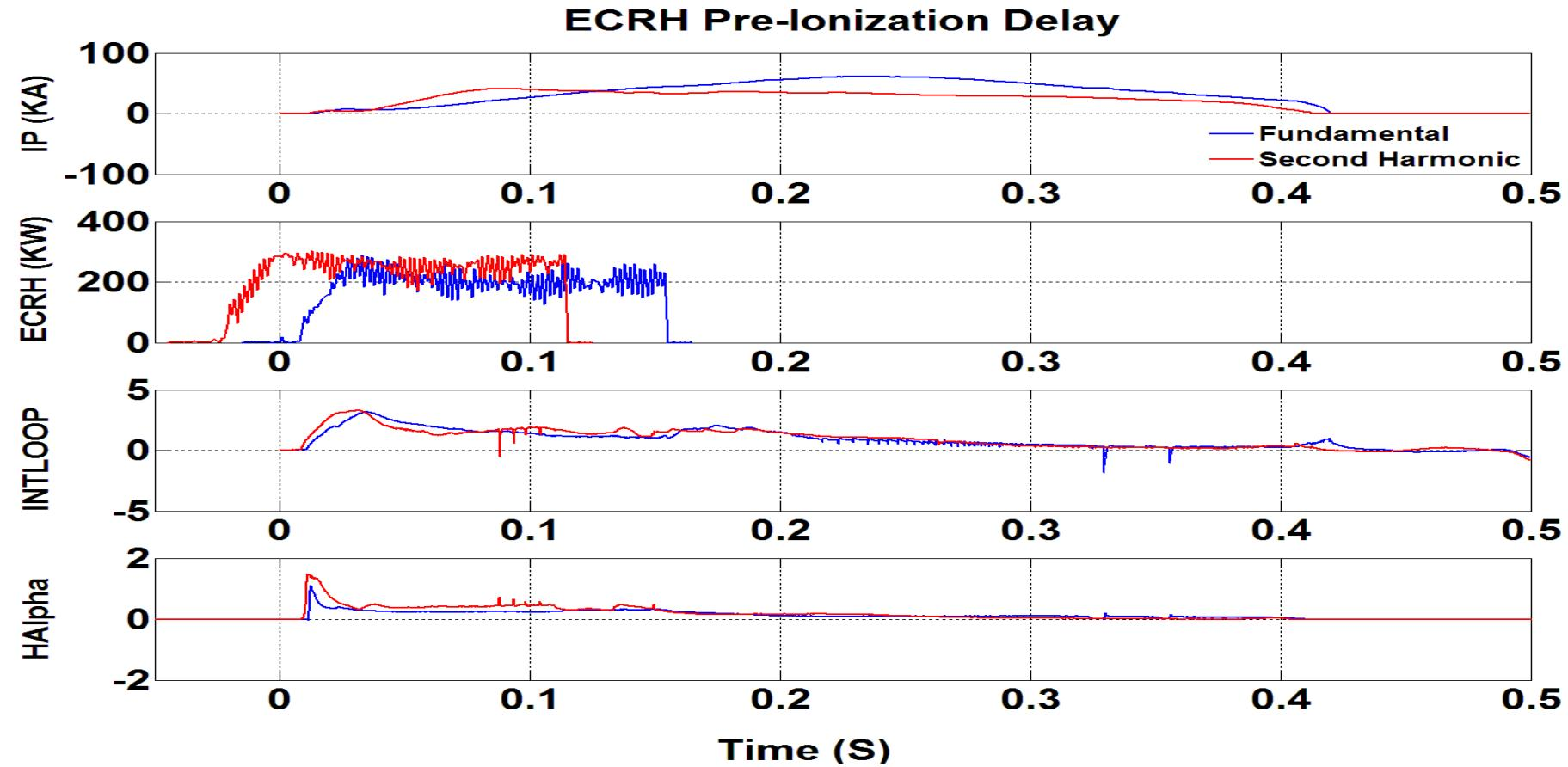
SST-1 operates successfully with both fundamental and second harmonic ECH pre-ionization with loop voltages ~ 3 V
