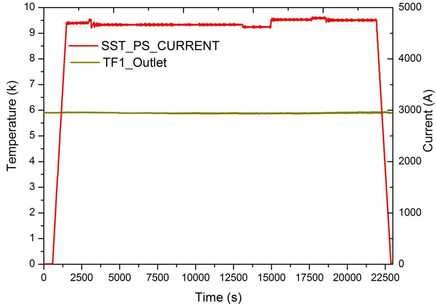
Established long duration Superconducting Magnet operational scenarios
