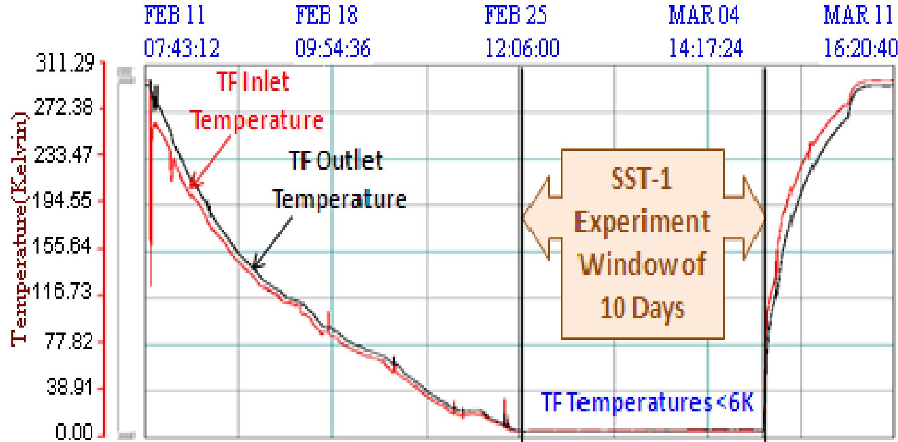
Established the appropriateness of helium refrigerator towards thermal stress optimized cooling down of the cold mass
