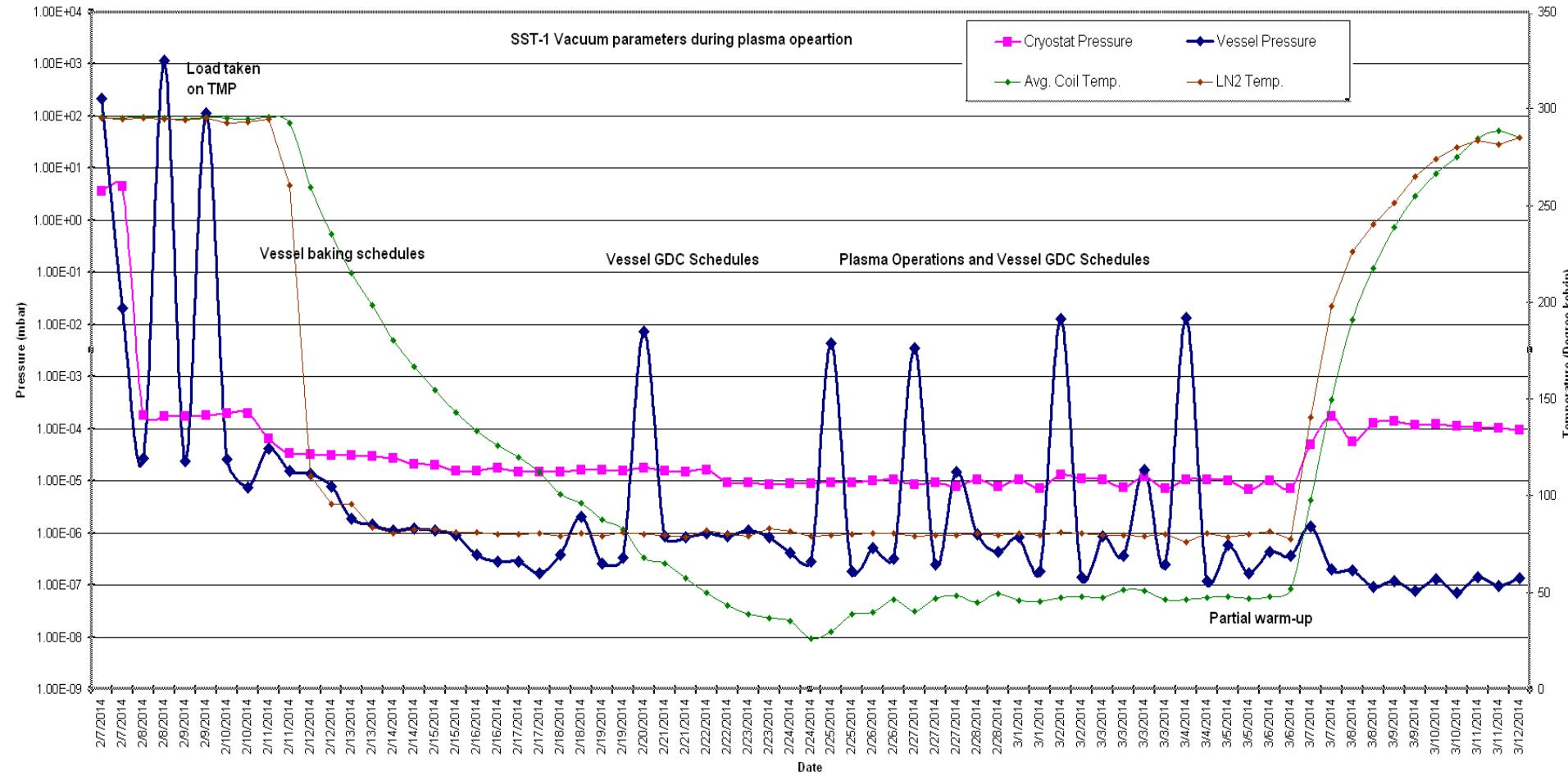
Established UHV compatibility of SST-1 Vacuum Vessel, baking compatibility with 80 K shields being maintained
