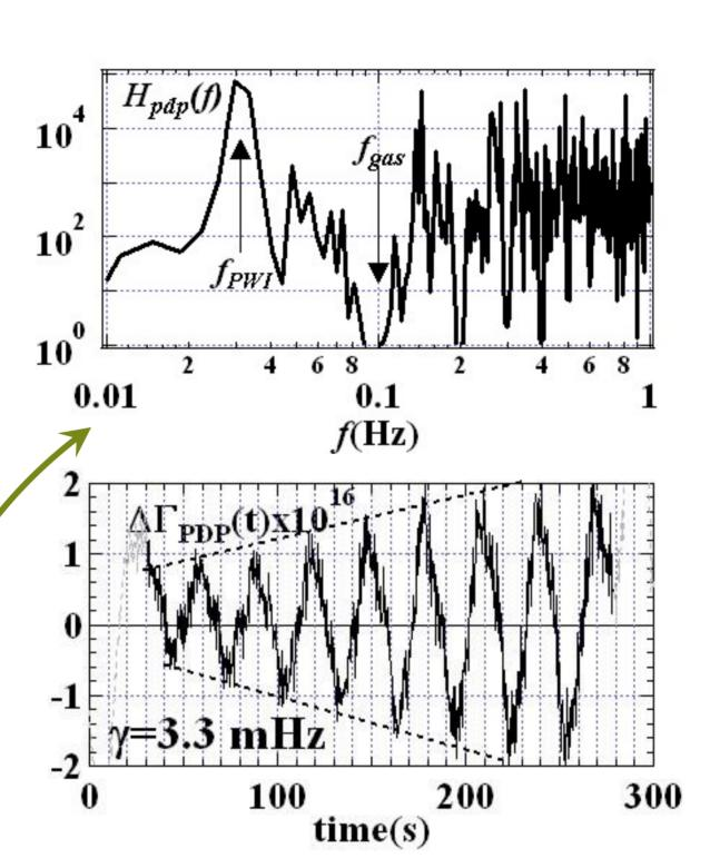
Frequency response function  $H_{pdp}$  to  $H_2$  puff in vacuum. Arrows indicate  $f_{gas}$  and  $f_{PWI}$ . Minima for  $f>f_{gas}$  in H(f) correspond to hamonics of  $f_{gas}$ . (b) The amplitude of  $\Delta\Gamma_{pdp}$  at  $f_{PWI}$  grows with a time constant of 3.3 mHz, which causes non-stationary particle circulation.
