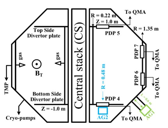
Major radius: 0.68 m Minor radius: 0.4 m PFCs surface ~ 35 m<sup>2</sup>  $T_{\text{wall}} \sim 100^{\circ} C$  $\tau_{pump} = 2 \text{ sec}$
