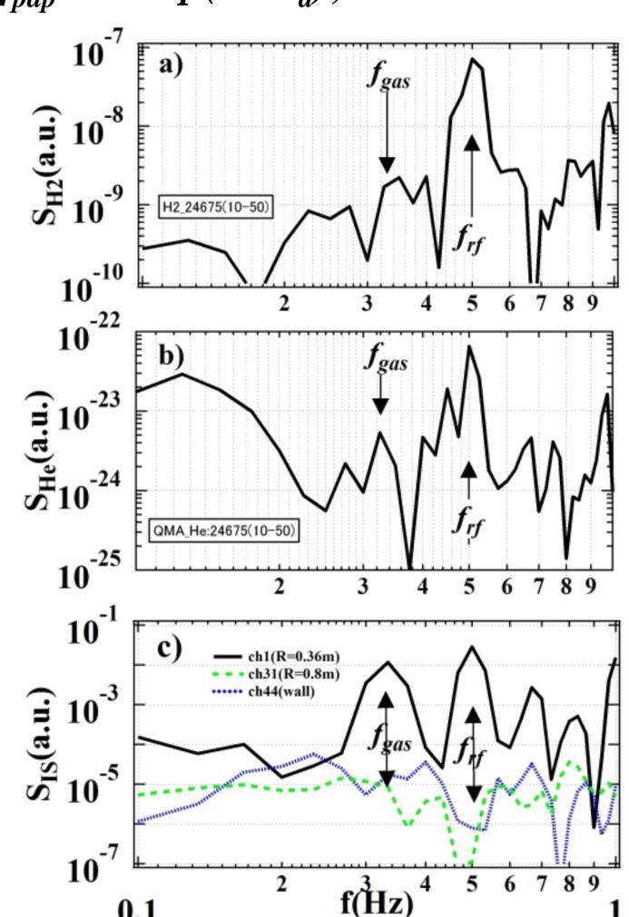
Auto power spectra (a)  $S_{H2}(b) S_{He}$  and  $S_{Is}$ are plotted.  $f_{gas}$  and  $f_{rf}$  are 333mHz and 500mHz, respectively.  $S_{Is}$  at R=0.36, 0.8m and the side wall are shown.
