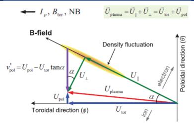
Apparent poloidal velocity is induced by the plasma toroidal and poloidal motion.
