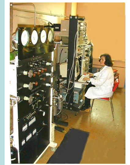
Fill System: Filling of CH shells with gaseous fuel up to 1000 atm at 300K
