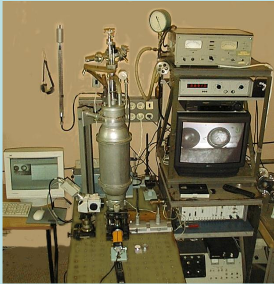
Cryogenic targets: FST method for fuel layering inside free-rolling targets
