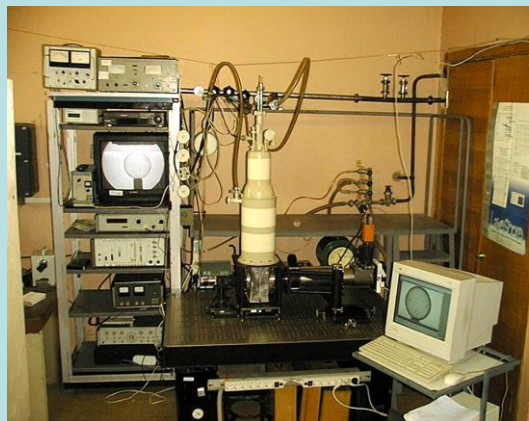
Cryogenic target characterization: 100-projections visual-light tomograph with 1 \mu\text{m} space-resolution
