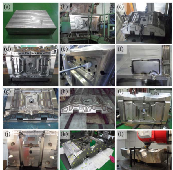
Fig. 2 Overall machining processes for manufacturing of the SB #8 FSP
