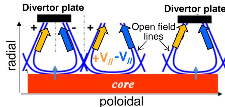
$$\triangleright \perp \text{loss of } //\text{-Momentum} \quad \frac{\tau_{m//}}{\tau_{m\perp}} = \frac{D_\perp L_{//}}{V_{//} \lambda_m^2} \propto f_{m0}$$
