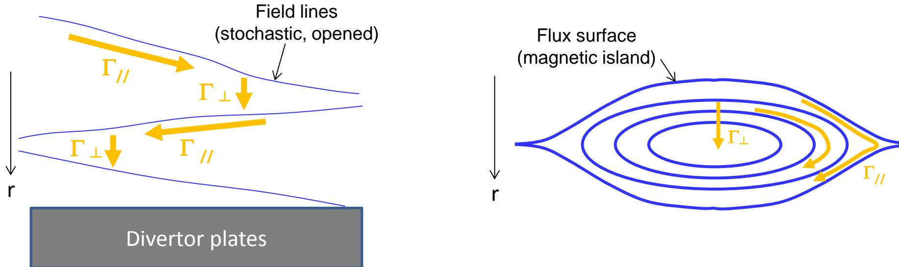
$$\frac{B_r}{B_t} = 10^{-4} \sim 10^{-3} \quad \frac{\Gamma_{//}}{\Gamma_{\perp}} = 10^5 \sim 10^8$$
