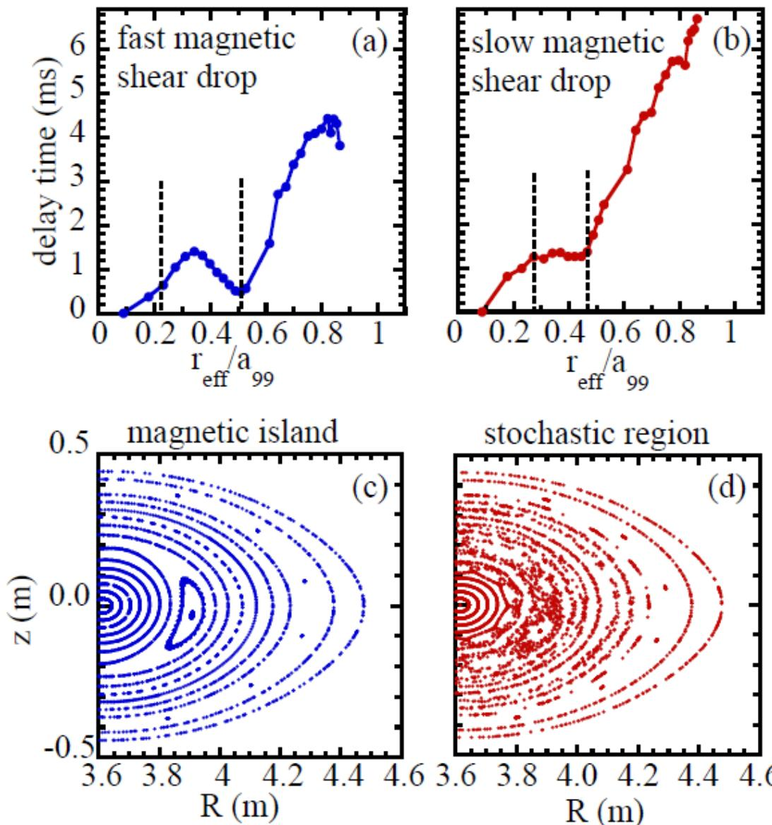
The time delay of heat propagation changes depending on the magnetic topology:
