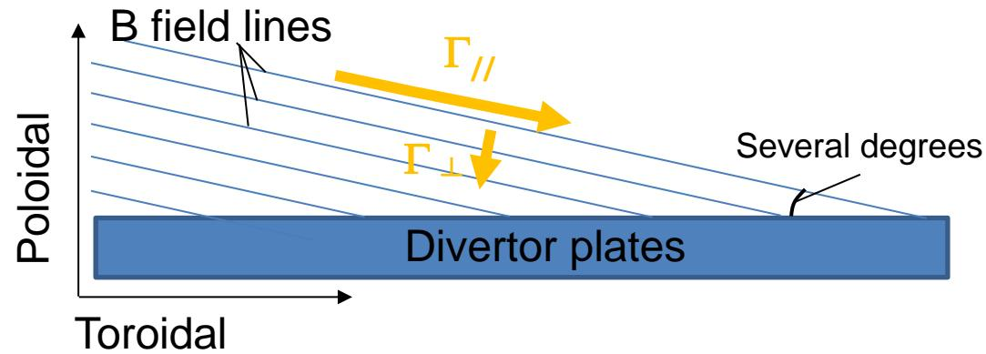
$$\frac{B_\theta}{B_t} \sim 0.1 \quad \frac{\Gamma_{\parallel}}{\Gamma_{\perp}} = 10^5 \sim 10^8$$
