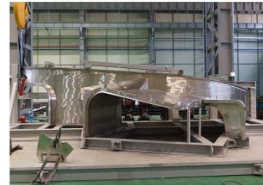
Full scale mock-up of VVTS 10 degree section
