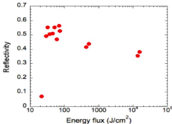
Figure 2: Plasma Mirror reflectivity versus laser energy fluence.
