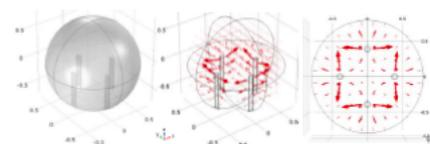
**Measurement and modeling of the ElectroMagnetic Perturbations** have been performed for ABC. Two types of antennas have been used: *SuperWideBand* (SWB) microstrip antenna, and commercial (GA.107 model by Taoglas) multiresonant monopole (WM). The ABC vacuum chamber was simulated with a COMSOL solver as a resonant cavity and as a non hollow cavity.
