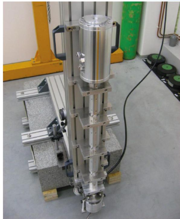
**1 meter long segment of the gas-acceleration section of the injector assembled**
