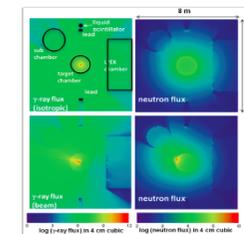
Fig. 1. Calculated  $\gamma$ -ray (left) and ( $\gamma$ ,n) neutrons (right) flux map around the target chamber for isotropic (top) and beam-like (bottom)  $\gamma$ -ray sources with  $10^{12}$   $\gamma$ -rays from the target at the center of the target chamber.
