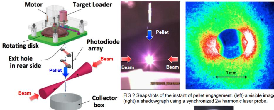
FIG.1 pellet injection and laser synchronous system
