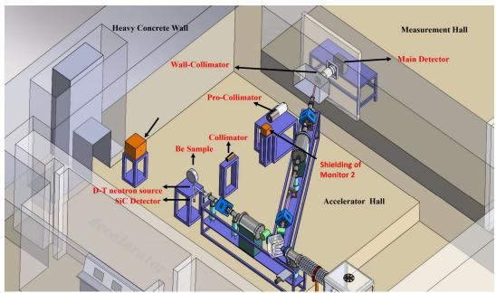
Measure TOF spectra of leakage neutrons at >90°.
