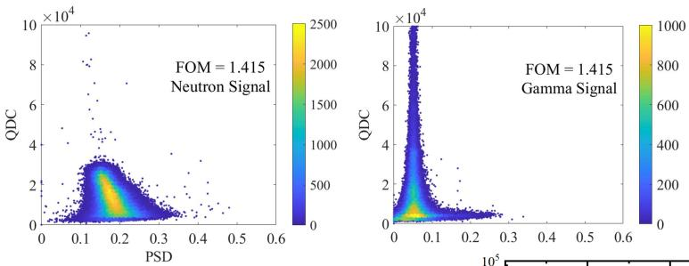
99.97% of all waveforms are distinguishable. The lower limit of distinguishable energy has been reduced from 150 keV to 70 keV. Waveform utilization rate has increased from 60% to over 99%.
