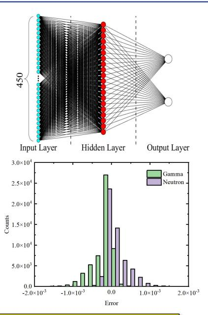
A single layer of 20 neurons yields optimal performance, with 99.9% particle confidence error below 0.02 and 100% discrimination accuracy.
