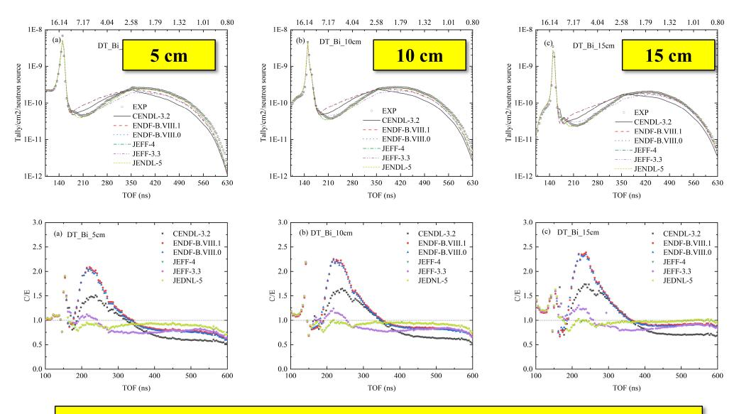
Experimental results at different thicknesses using a D-T neutron source, with point-by-point C/E comparisons against multiple nuclear data libraries.
