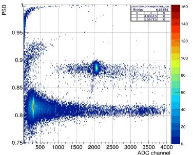
Li doping enables low-energy neutron detection, while chlorine (Cl) doping provides fast-neutron sensitivity via the <sup>35</sup>Cl(n,p) reaction.
