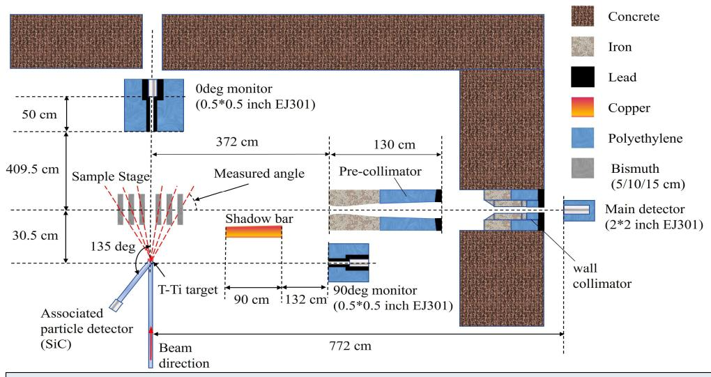
Neutron leakage spectra were measured for Bi samples of three thicknesses  $(5/10/15 \times 30 \times 30 \text{ cm})$  at six scattering angles  $(47^{\circ} /58^{\circ} /73^{\circ} /107^{\circ} /122^{\circ} /133^{\circ})$ .
