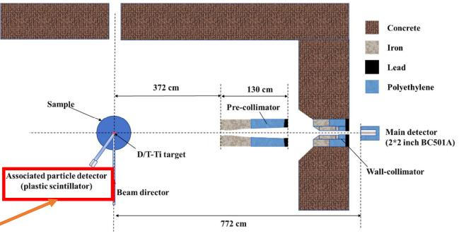
Because the sphere fully enclosed the target head and disabled the monitor system, the pulse time distribution was determined using the associated-particle detector.
