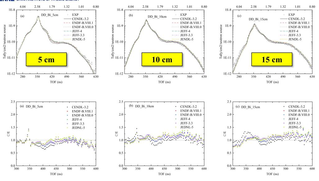
Experimental results at different thicknesses using a D–D neutron source, with point-by-point C/E comparisons against multiple nuclear data libraries.
