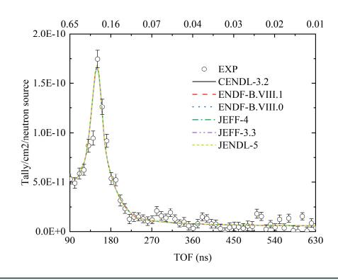
A 12 cm-diameter polyethylene sphere was used as the benchmark sample to validate the platform, with C/E deviations < 5% across libraries.
