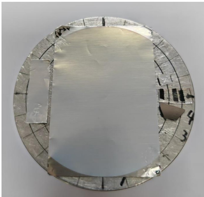
Sample for Rutherford backscatter (Cropped \text{C}_3\text{H}_6\text{N}_6 target)
