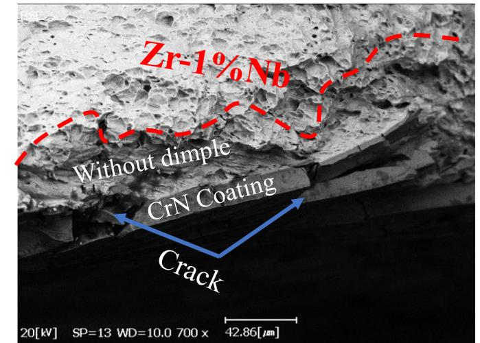
Fracture surface of CrN-coated Zr-1Nb cladding tube
