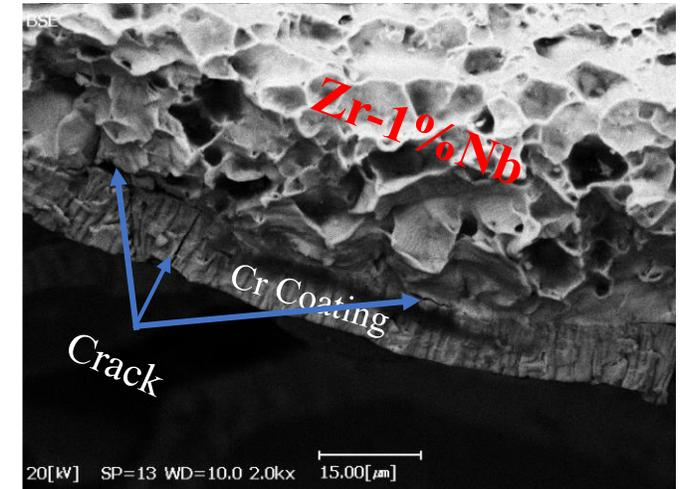
Fracture surface of Cr-coated Zr-1Nb cladding tube
