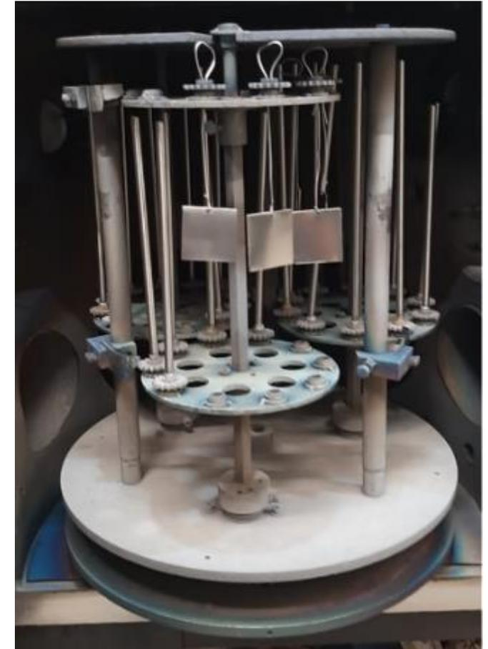
The inside view of the ARC-PVD coating chamber.
