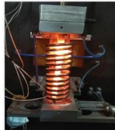
High frequency induction furnace (180 kHz)
