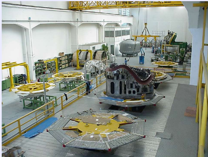
Winding of Coil Types 2, 3 & 4
