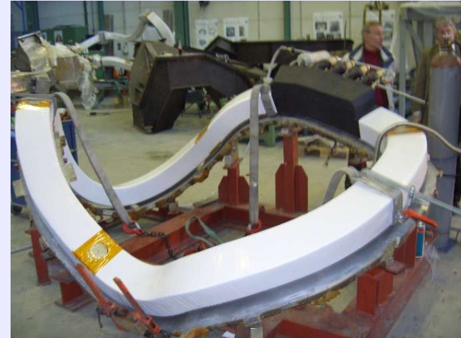
Winding of Coil Types 1 & 5
