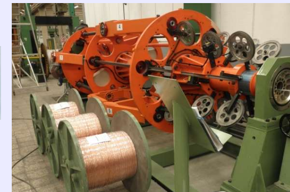
Final stage cabling machine
