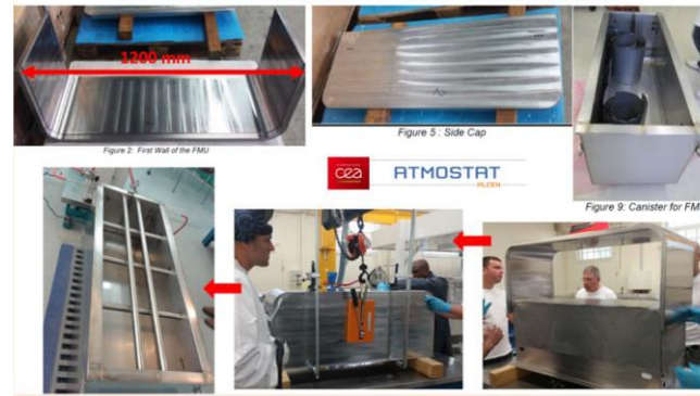
FW and 2 SC assembly by 2-step HIP process (EUROFER97)
