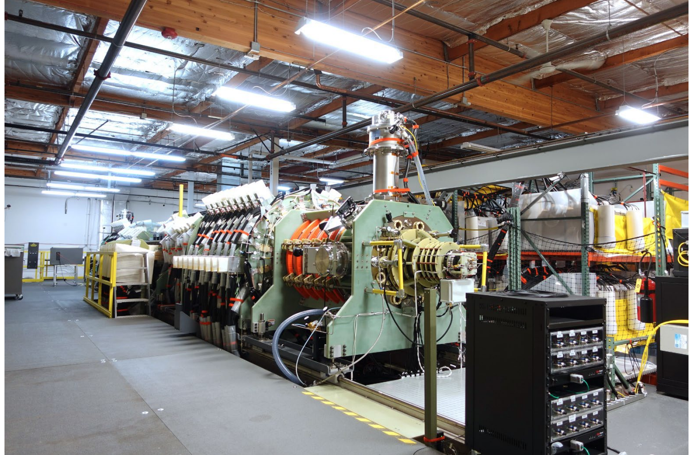
Trenta, Helion's 6 th fusion prototype
