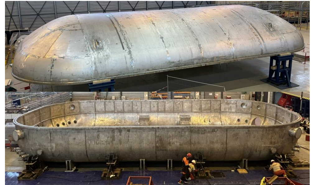
Cold Test Facility for TF Coils (4K / 68kA)
