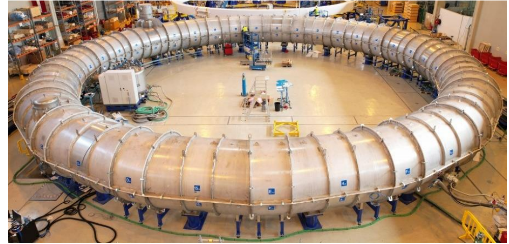
Cold Test Facility for TF Coils (4K / 68kA)
