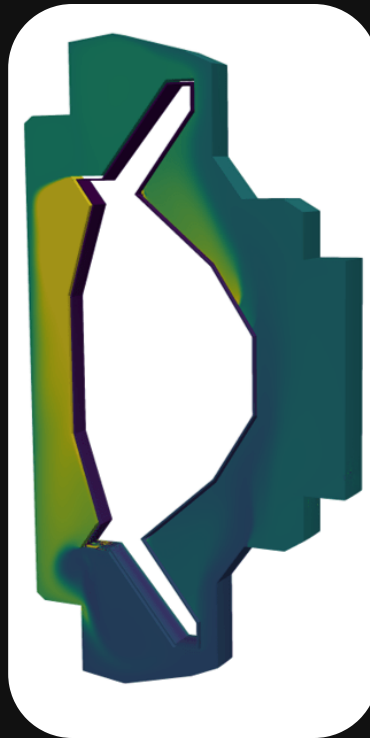
FESTIM model of an ARC's breeding blanket
