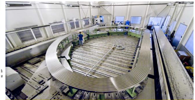
The radial plates that hold the conductor of the toroidal field coil: D-shaped stainless steel structures with grooves machined on both sides along a spiral trajectory.
