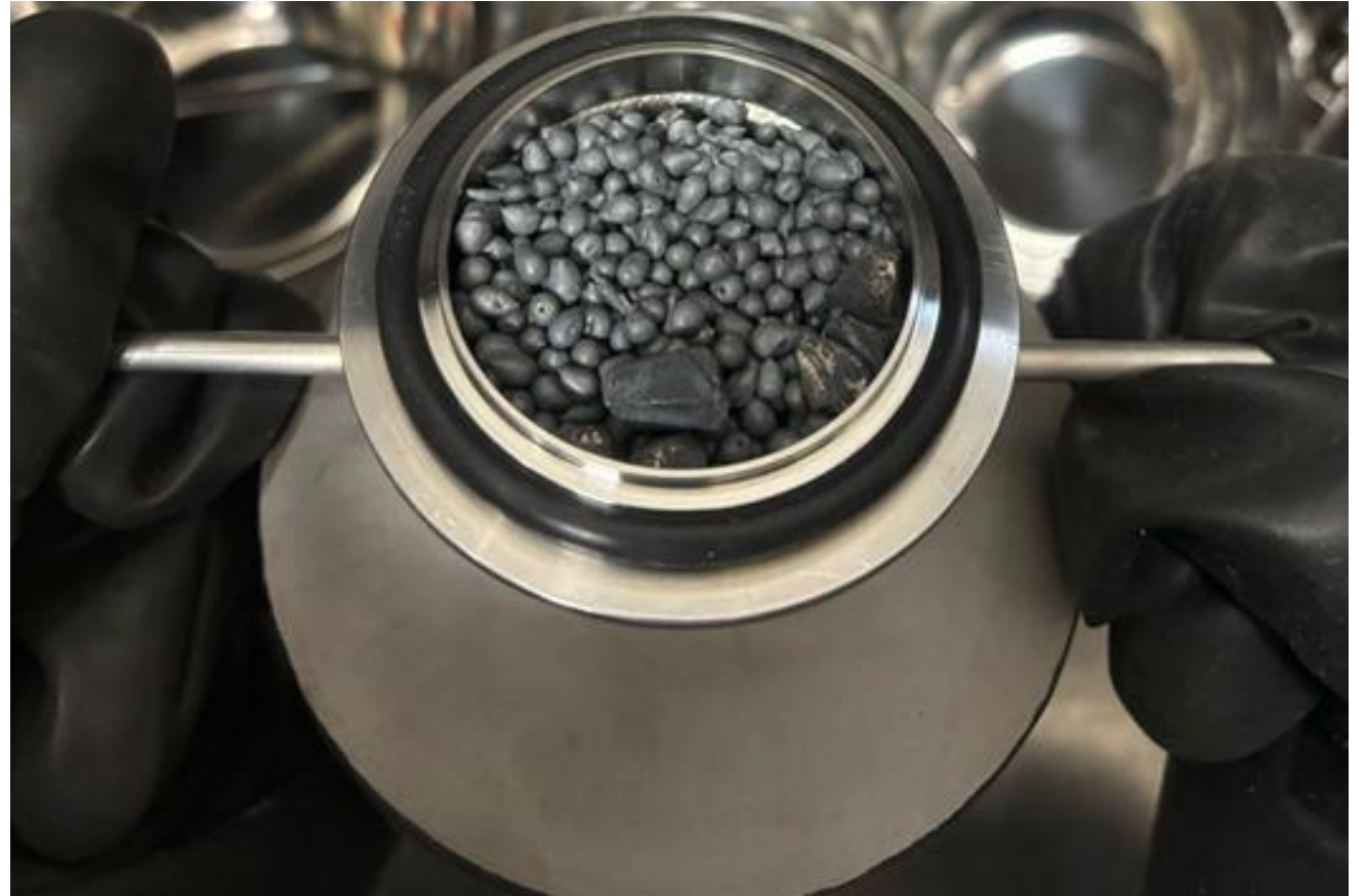
Condition after loading the crucible with raw materials (400 cc)
