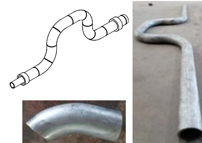
Forming of double-layer pipe assembly mockup
