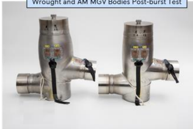
Wrought and AM MGV Bodies Post-burst Test
