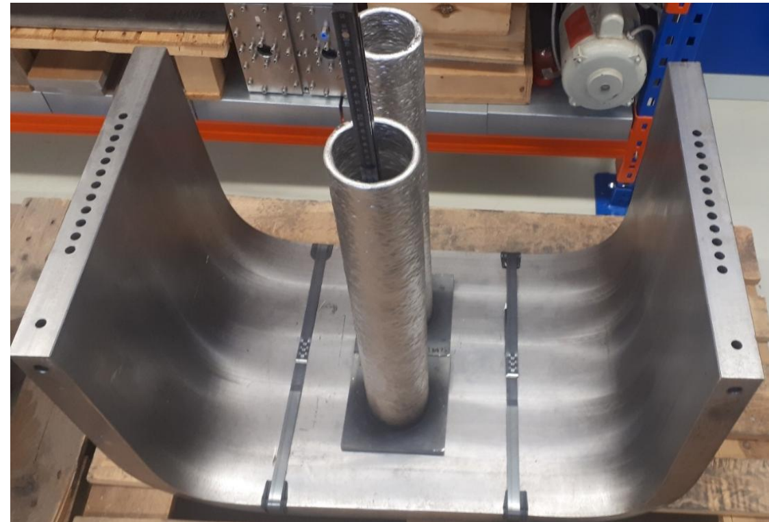
Pressure Tubes via WEBAM on U-shaped FW Mock-up
