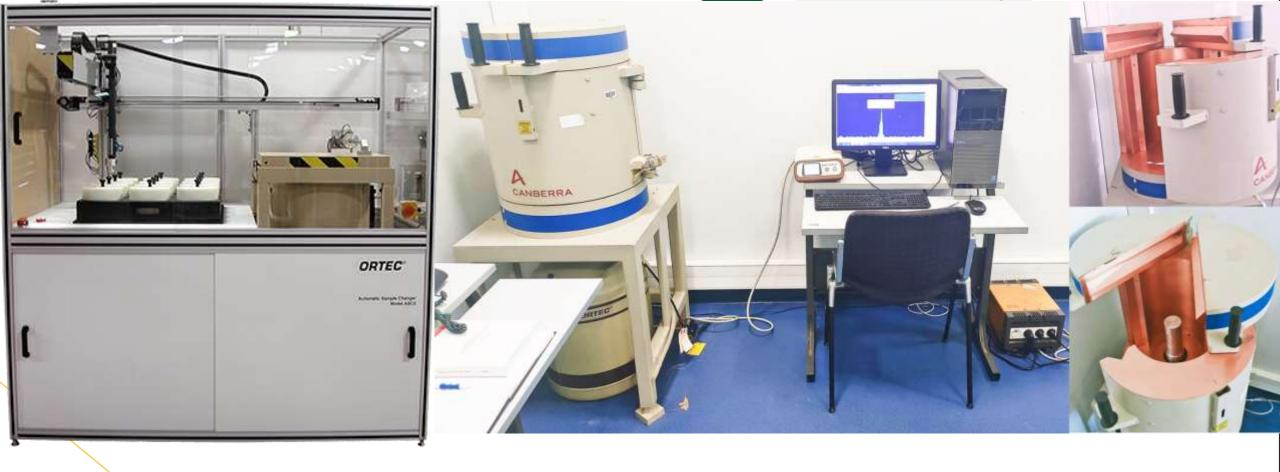
03 Vertical HPGe P-type Detector with 30% Relative efficiency (FWHM=1.85 keV)
