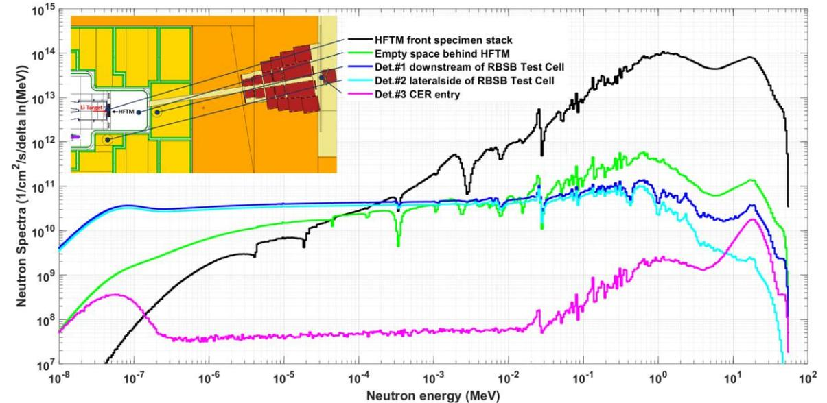
Neutron flux spectra at different location of test cell
