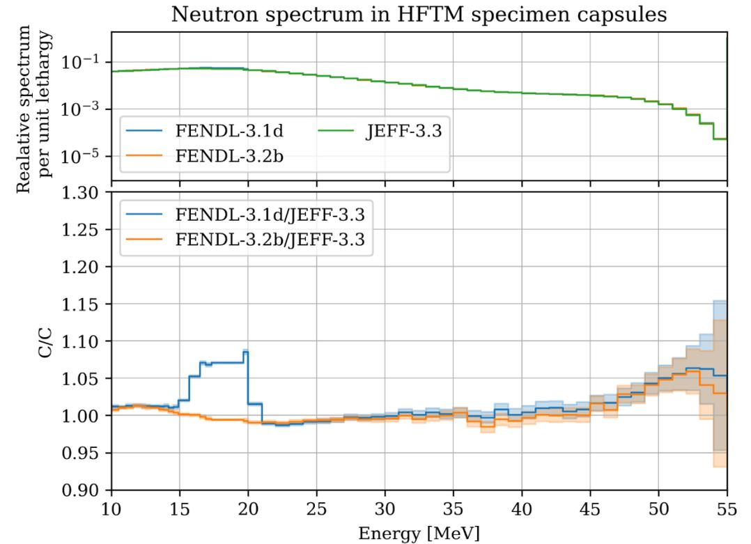
High Flux Test Module
