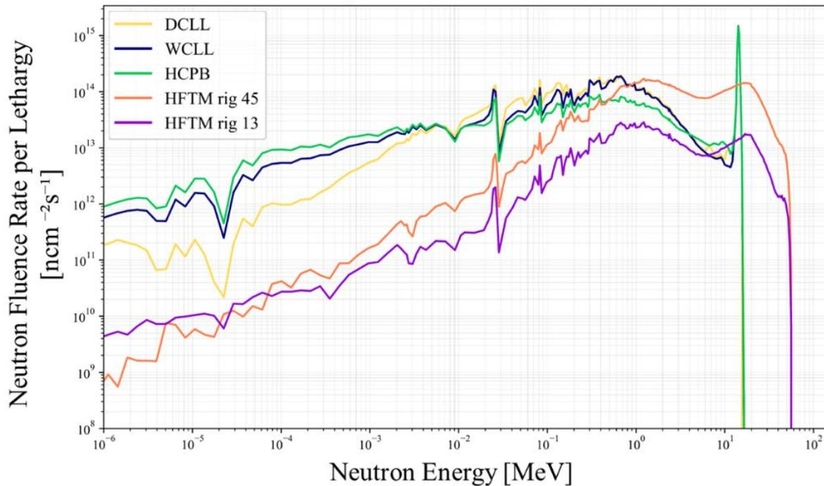
Neutron flux spectra comparison with DEMO blanket
