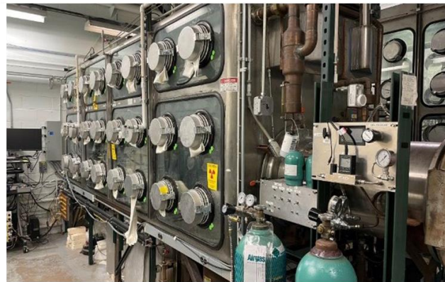
LSTL - Liquid Salt Test Loop at ORNL FLiNaK – 700C 80L
