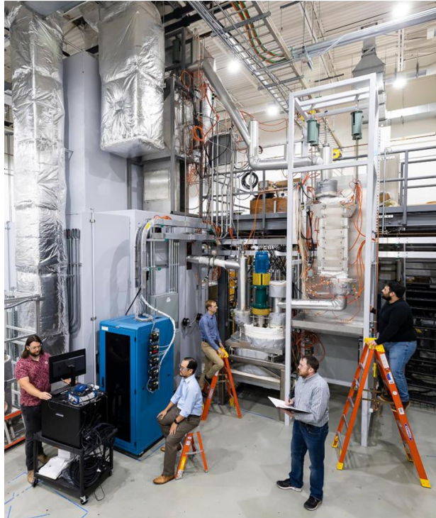
FASTR - Facility to Alleviate Salt Technology Risks – ORNL NaCl-KCl-MgCl 2 725C 154L
