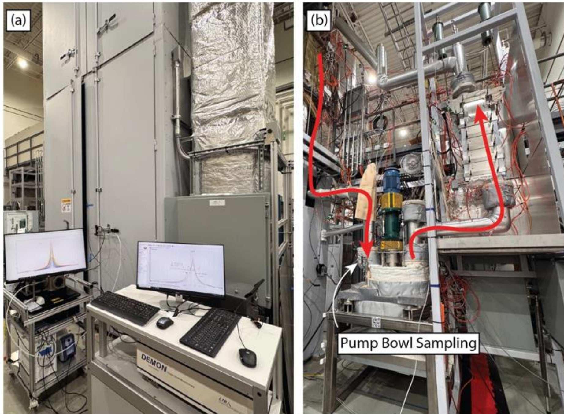
(a) FASTR storage tank with LIBS cart in the front left and DEMON spectrometer in the front right.
