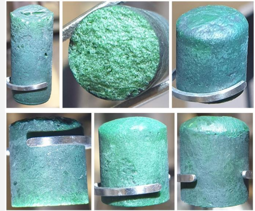
Final ingots of fuel for SALIENT-03 irradiation experiment
