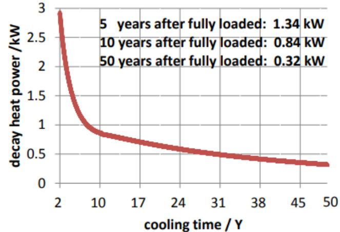
Fig. 6: Spent fuel canister decay heat power in
