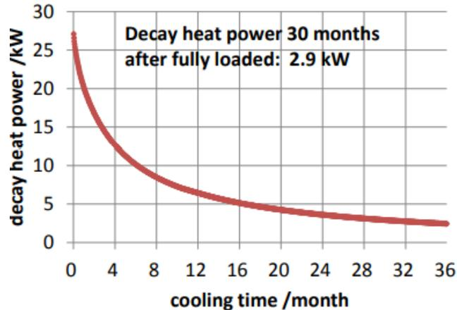
Fig. 5: Spent fuel canister decay heat power in
