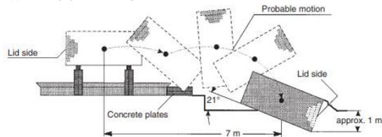
Figure 13. Movement of the CASTOR cask after the impact of the propane rail tank explosion.
