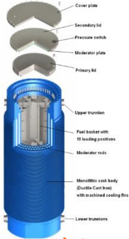
CASTOR<sup>®</sup> casks fulfil all protection objectives during transport and dry interim storage
