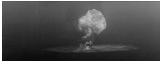
Figure 7. BLEVE, expanding fireball, photographs taken from a helicopter.
