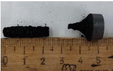
TRISO intact and graphite particles
