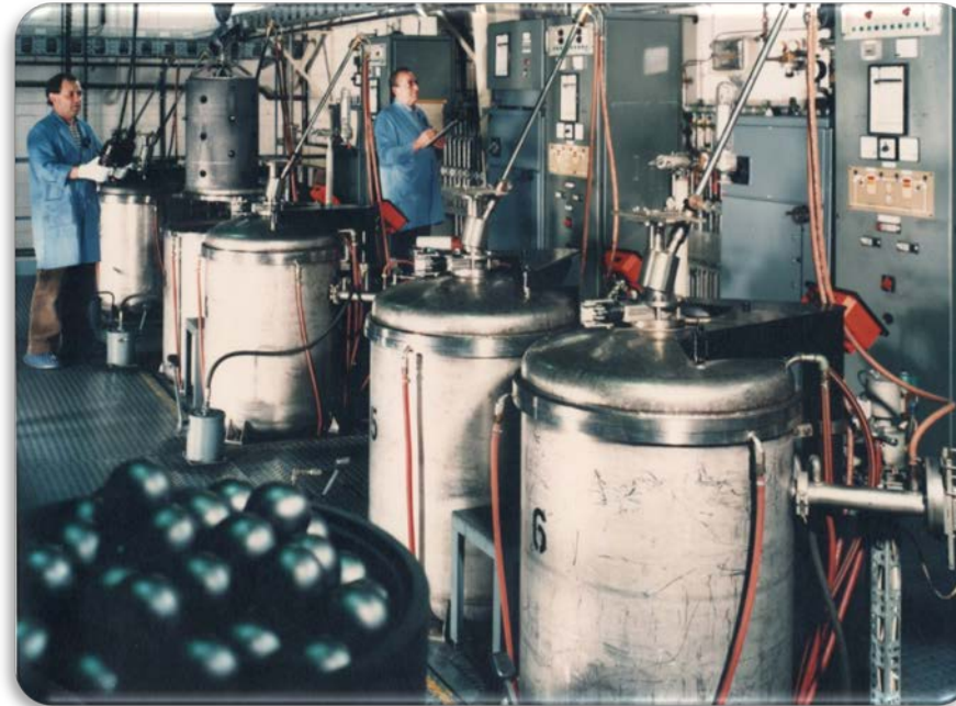
Fuel Sphere Pressing Line (NUKEM HOBEG, Hanau, Germany)
