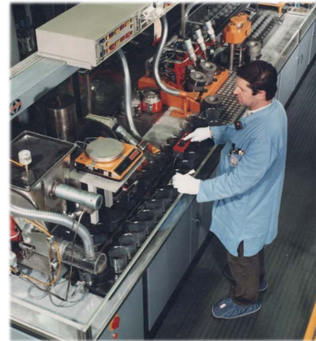
Fuel Sphere Pressing Line, (NUKEM HOBEG, Hanau, Germany)
