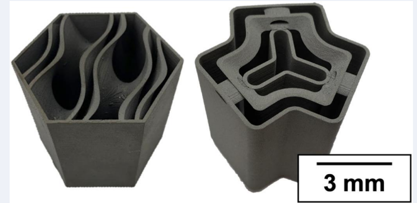
Examples of fuel compacts fabricated containing coolant flow channels and particle zones using 3D-printed SiC
